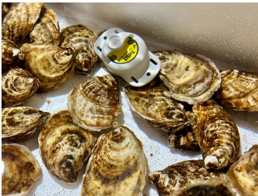
Figure 2. Water temperature monitored using an Onset HOBO Tidbit MX2203 logger.
